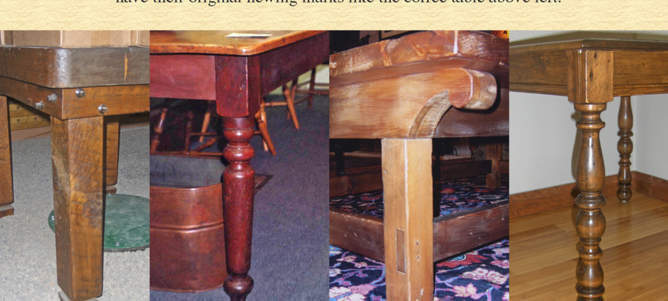
Legs - from left to right; cut from a beam keeping all the mill marks, a reused set of original old legs, reclaimed wood milled smooth then antiqued, a new Jacobean turned leg from reclaimed barn floor boards.
